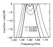
Fig. 2. Characteristics of mode splitting (meander loop: a = 16 mm, b = $3.25 \text{ mm}, w_1 = 2 \text{ mm}, w_2 = w_3 = s = 1.5 \text{ mm}$ ).
