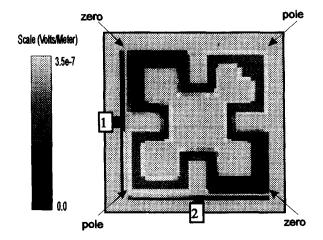
Fig. 3. An electric field pattern of the dual-mode microstrip meander loop resonator
